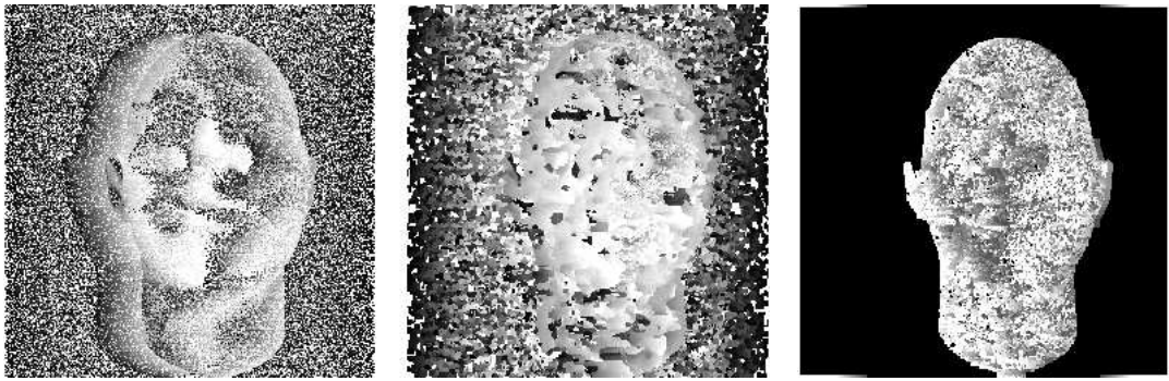
Figure 27: Disparity maps for pixel intensities and normals and mean curvature for uniform noise of 20
